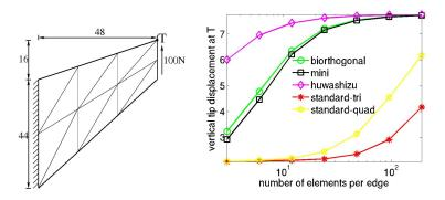
Cook's membrane problem with initial triangulation (left) and the vertical tip displacement versus number of elements per edge Note: Hu-Washizu and standard-quad are computed on quadrilateral mesh with the equal number of nodes.
